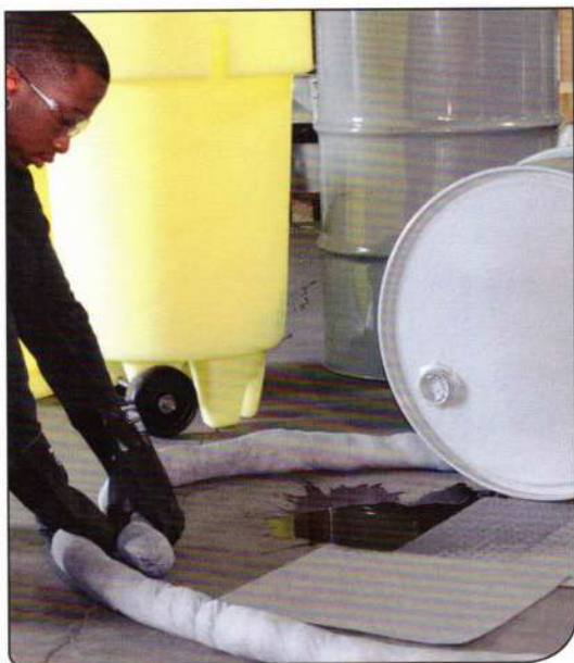
Kits strategically positioned throughout a facility provide fast, emergency response to dangerous spills.
