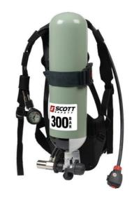
The SCBA consists of a back plate, carrying harness and pneumatic system, containing a reducer with integrated cylinder connector, pressure gauge, whistle and demand valve. It can be configured in a number of different ways with various sized single cylinders and the choice of Vision 3, Panaseal, Panavisor or Promask PP facemask.
